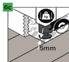
In the case of any heavy objects placed on the floor (such as kitchen furniture, kitchen island, built-in wardrobes and other furniture permanently attached to the wall), 5mm expansion joints should be left around them. We recommend the following ways to preserve expansion joint spaces:
