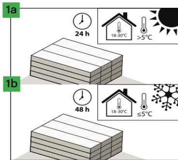
If the temperature is  $>5^{\circ}\text{C}$  during transport, the acclimatization time in a room with a temperature of  $18-30^{\circ}\text{C}$  should be min. 24 hours. However, in case of temperature  $\leq 5^{\circ}\text{C}$  during transport, acclimatization time in a room with a temperature of  $18-30^{\circ}\text{C}$  should be min. 48 hours.
