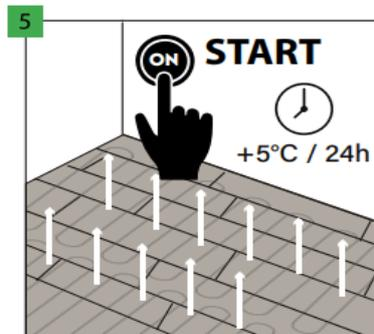
After laying the floor and waiting 24 hours, you can turn on the underfloor heating, remembering to gradually increase the temperature (5°C per day). ATTENTION! It should be remembered that the maximum temperature of the floor surface is 27°C.
