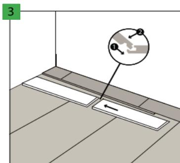
The floor panels are provided with locks on the short and long side. First, join the short sides of the neighbouring panels together.
