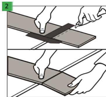
For additional cutting of floor panels, use a sharp knife, cut the top layer, then break the panel dynamically by leaning it on the edge. The floor panels may also be easily cut using an electric saw.
