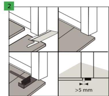
Expansion joints along the walls must be covered with a decorative strip, assembling it by means of glue or special clips. It is recommended to use the Arbiton strips dedicated to a given panel, which guarantee the excellent colour match and the coat resistant to scratching.
