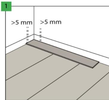
Leave 5 mm of perimeter space at the walls to allow the floor expansion. The maximum surface which can be laid without additional expansion joints is 200 m<sup>2</sup>. Above this surface, apply an additional expansion joint and enlarge all the expansion joints up to 10 mm. The maximum length of the floor surface in one direction, which can be laid without additional expansion joints is 20 m. Above this length, apply an additional expansion joint and enlarge all the expansion joints up to 10 mm.
