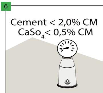
In the case of the cement grout, the moisture content in the substrate must be lower than 2.0%, and in the case of the anhydrite grout, it must be lower than 0.5%. In the case of installation with the underfloor heating, the abovementioned values must be 1.8% and 0.3% respectively.
