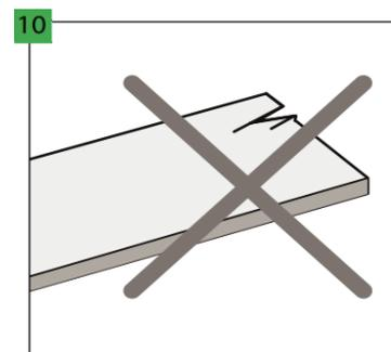
Before and during the installation, control all the panels in the optimal lighting conditions. Do not use defective panels.
