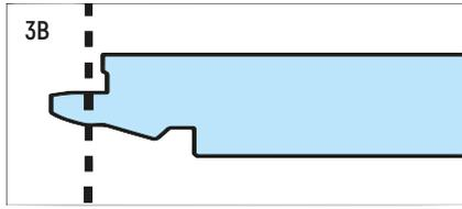
Begin the first row with a whole plank. First saw off the tongue on both the long and the short sides. (See diagram 3B.)
