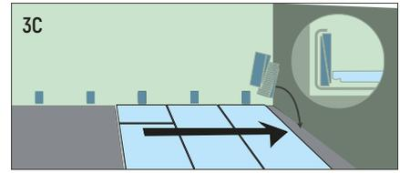
Put the plank with the sawn off sides against the walls. Put spacers from the installation kit between the planks and the wall. This will ensure that your expansion joint is wide enough: 8 to 10mm [5/16" to 3/8"]. (See diagram 3C.)
