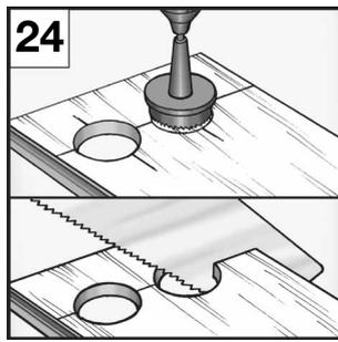
For heating-radiator pipes, holes that are drilled 3 cm / 1.2" larger than the pipe diameter must be avoided. A "fitting piece" should be cut out, glued, fitted in and fixed in place with a wedge until the glue has dried. Then cover the recesses with a radiator-sleeve [23, 24, 25].
